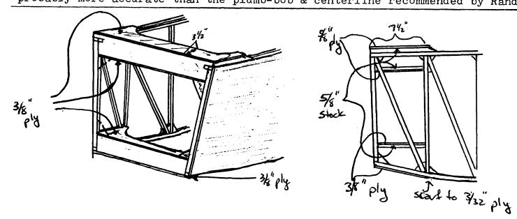
Here are a couple of rough sketches of the modifications I made to the firewall of my KR-1 as a beef-up to take a larger VW than Rand used on his prototype. I plan to start out with a 1600cc and later upgrade it to an 1834cc. This mod. is very light and very strong. I thought maybe some of the other KR-1 builders might want to use a similar set up. Mike Wray Tucson, AZ
