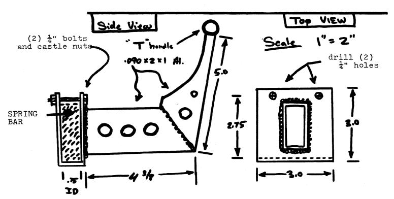
MATERIAL - Spring bar... 1/8" aluminum plate 2024-T3 heliarc welded, or.. use aluminum extrusion 2024-T3
