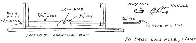
JO DRILL LOCK HOLE, CLAMP 3/4" BLOCKS TO BOTH SIDES WITH 1/8" PLY IN PLACE.
