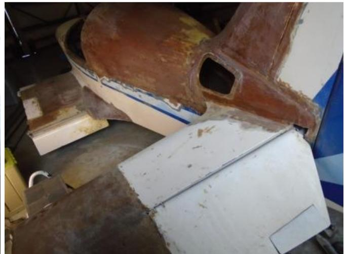
The horizontal stabilizer has been extended 6" on each end while the elevator has been shortened by 4" on each side as per Troy Petteway's aircraft for increased pitch stability. Vertical stabilizer has been enlarged and heightened with communication antenna molded inside. <http://www.n56ml.com/troy/>
