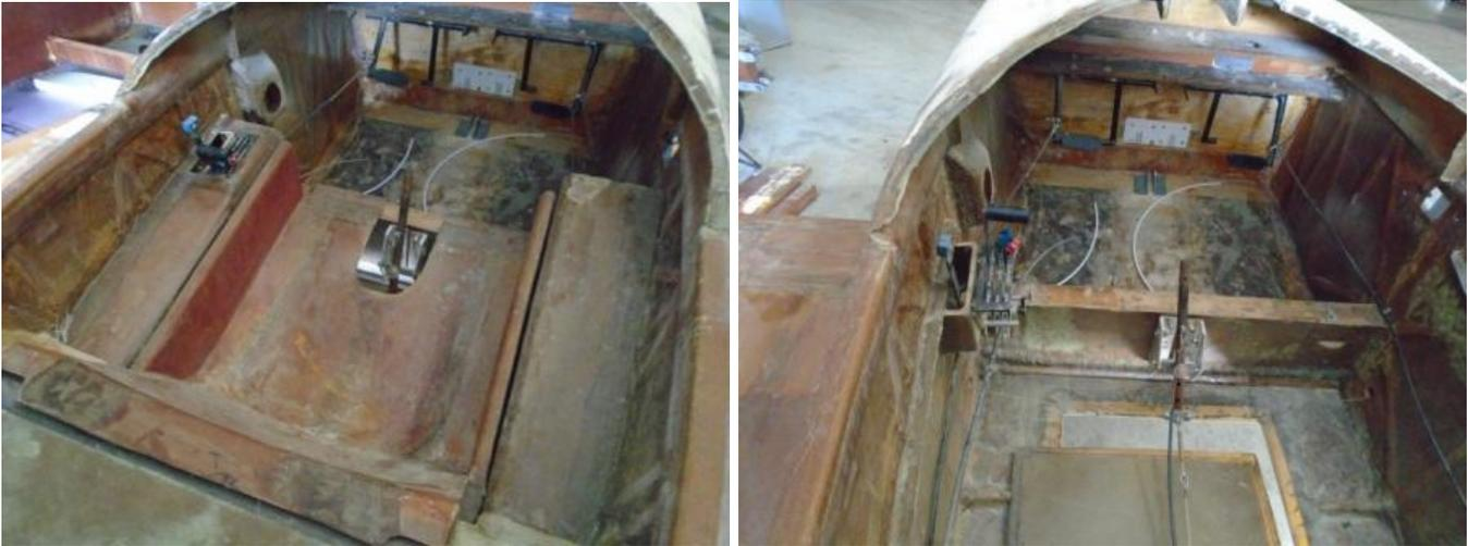
Fuselage, empennage and turtle deck have all been hardened with turtle deck heightened 8" to accommodate professionally molded single seat modification which is available complete with modified rudder pedals, side consoles and throttle quadrant if a roomier single place is desired instead of a comfortable 2 place configuration with standard rudder pedals. Belly access panel makes working in cockpit much easier and allows for better inspection capabilities.
