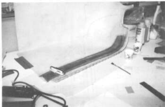
TWO (2) PLYS OVER PLYWOOD "INSERT". NOTE HINGE STRIP.
