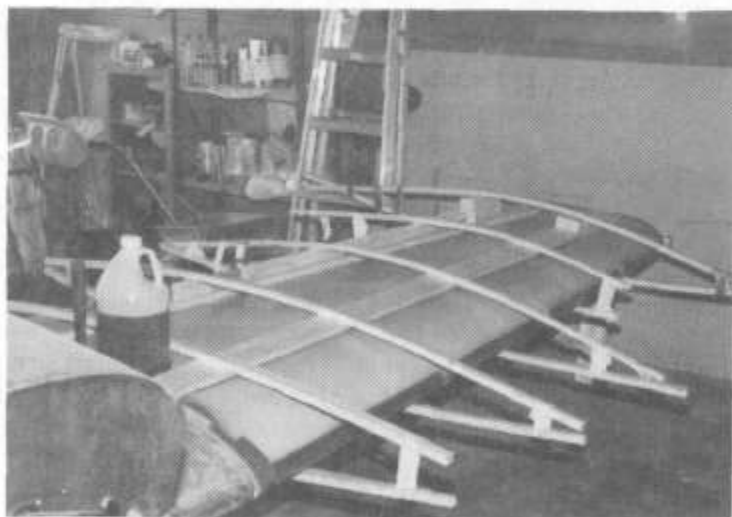
BOTTOM SKIN IN PLACE
