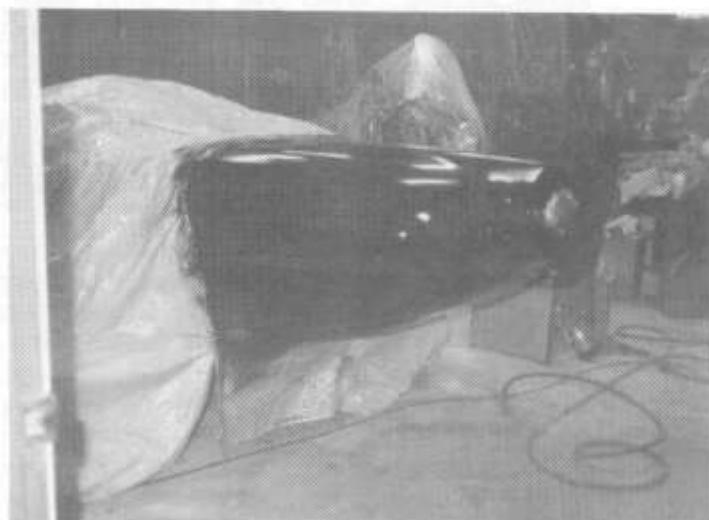
6. THE RAMANEL HARD SURFACE COATING AFTER SPRAYING.
