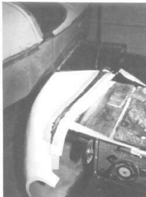
SINGLE FIBERGLAS OVERLAY ON EXTERIOR. COWL REQUIRED BEVEL SANDING TO BLEND IN FIBERGLAS PRIOR TO OVERLAY. LOWER HINGE STRIP VISIBLE. NOTE AMOUNT OF COWL DEPTH EXTENSION REQUIRED & ITS TAPER CUT.
