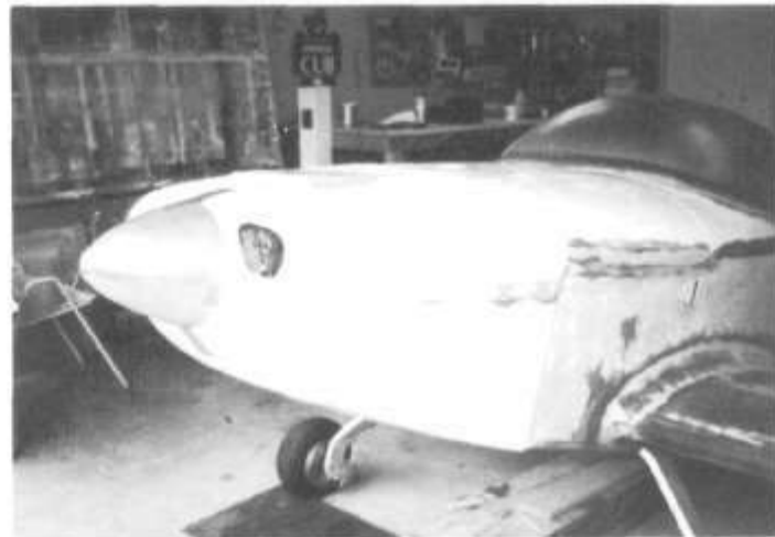
COWL ON. FIT & FILL IS MOSTLY COMPLETE EXCEPT FOR A CAMLOC ON COWL AT SPINNER LOCATION. NOTE THE OIL COOLER BUMP.
