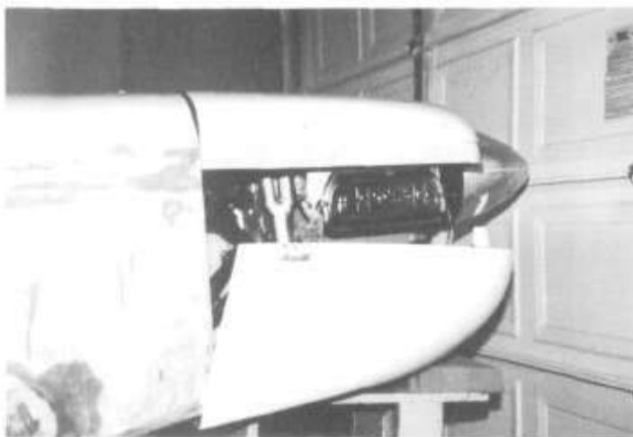
TOP COWL WITH HINGE STRIPS IN PLACE. LOWER COWL BEING BLOCKED INTO PLACE PRIOR TO AFT SKIRT TRIM.
