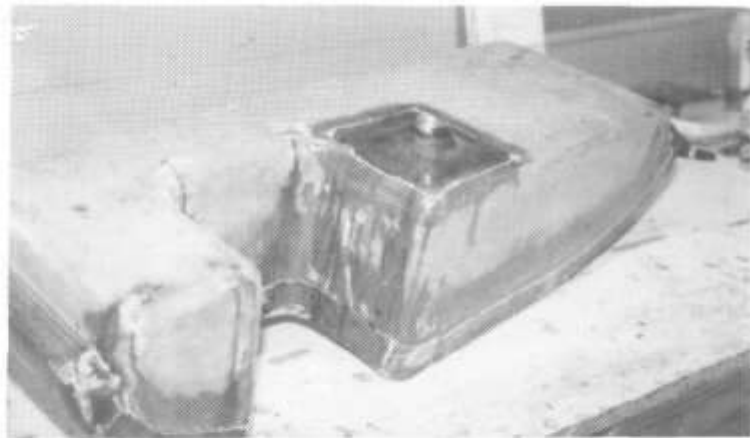
FIBERGLASSING TANK FLANGE
