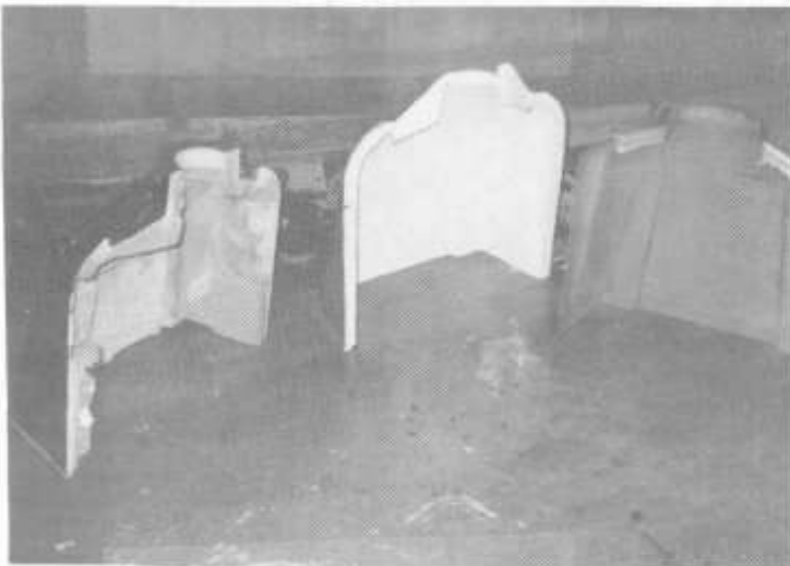
9. HERE ARE THE THREE STEPS IN MOLD MAKING. FROM LEFT TO RIGHT, THE PLUG, THE MOLD AND THE PART.
