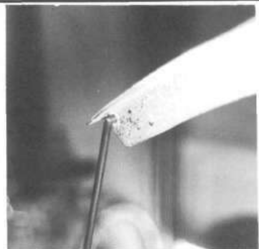
BRASS RECEIVER TUBE FOR CANOPY STAY IS FLOXED INTO THE WOOD PORTION OF CANOPY FRAME.
