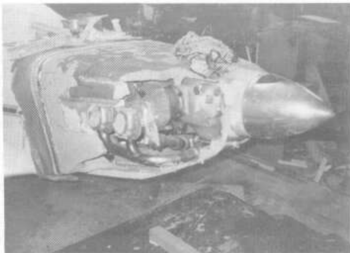
2. THE DISASTER! THIS IS WHAT WAS LEFT OF THE PLUG AFTER REMOVING THE IMPROPERLY CATALYZED RESIN AND GLASS.
