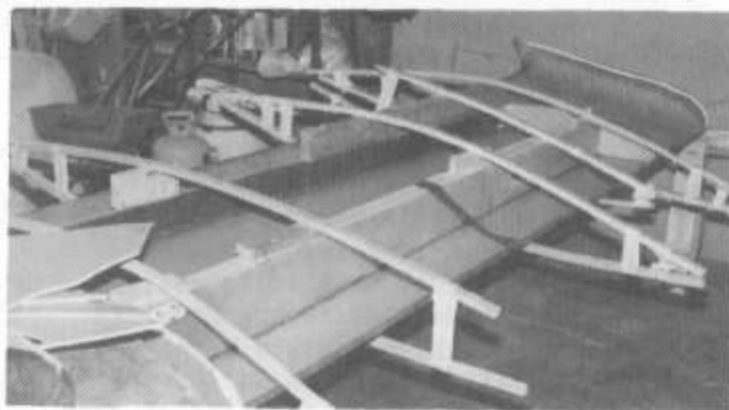
TOP SKIN CLAMPED IN PLACE
